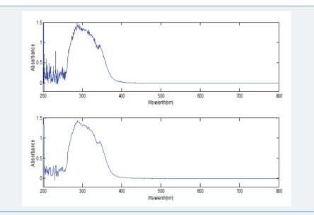
Figure 4: The UV spectrum of the eluent liquid before smoothing (above) and after smoothing (below).
