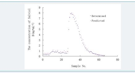
Figure 7: The predicted concentration of Salviol B by stepwise regression model using UV spectral data and the determined concentration of Salviol B using HPLC.
