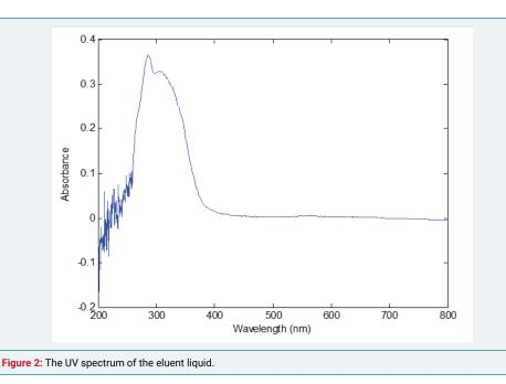
Three batches of samples were collected from the production line. The time interval was 5 minutes between two samples collected from the eluent liquid of the macroporous resin chromatographic column. In addition all the samples were diluted according to the ratio 1:200 with water before scanned with the portable spectrometer.
